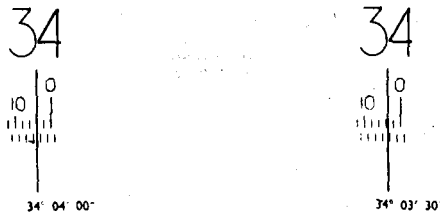
FIG. 391.—SYSTEM OF HORIZONTAL CIRCLE READINGS ON C. T. & S. OPTICAL SCALE THEODOLITE NO. IV.
